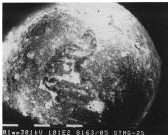
Fig. 2. Granule lubricated by 2% magnesium stearate. \times 80 .
